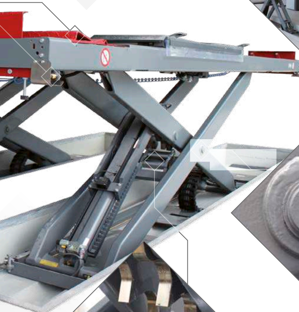
The cylinder raising support with step lever and rollers conducts a pure rolling movement. No sliding movement between the moving parts, meaning it is low noise, wear resistant and nearly maintenance-free.
