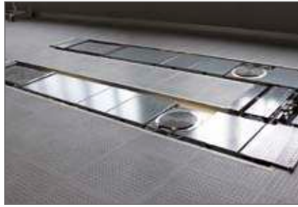
DUO CM in strip foundation (equipped for wheel alignment).
