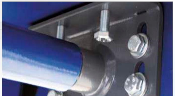
Adjustable bearing enables independent alignment of runway to scissors.
